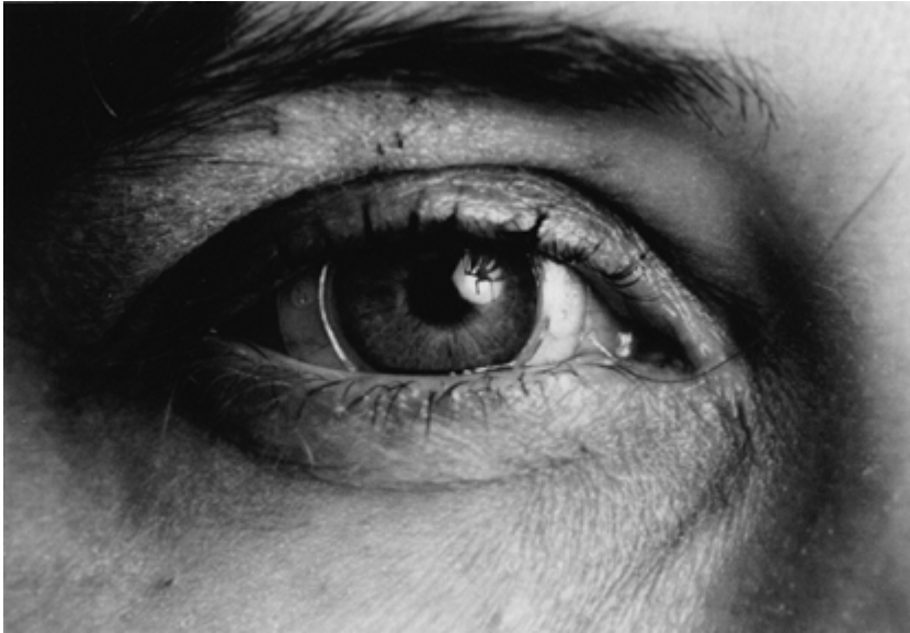
Figure 23.2. A method for precise measurement of horizontal, vertical, and torsional eye rotations. The subject is wearing a Silastic © annulus embedded in which are two coils of wire, one wound in the frontal plane (to sense horizontal and vertical movements) and the other effectively in the sagittal plane (to sense torsional eye movements). When the subject sits in a magnetic field, voltages are induced in these search coils that can be used to measure eye position. (From Leigh RJ, Zee DS. The Neurology of Eye Movements . Ed 3. New York, Oxford University Press, 1999.)
